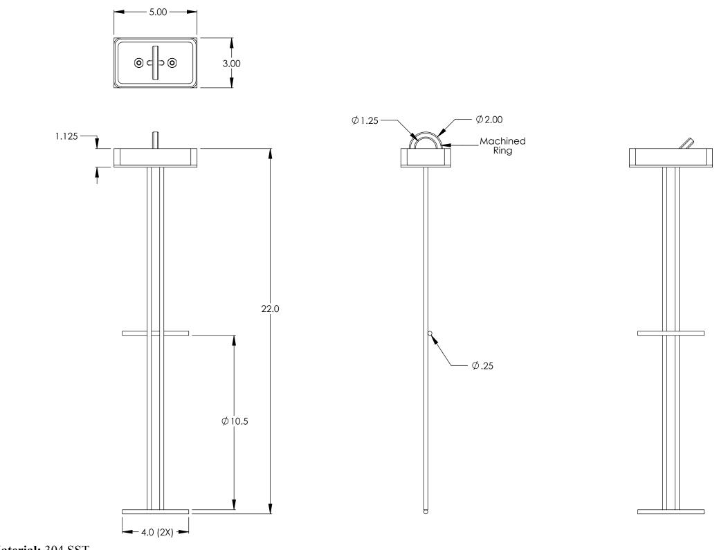
Material: 304 SST Work Load: 2000 lbs Configurations: With or without cover Manufactured: Minnesota, USA
