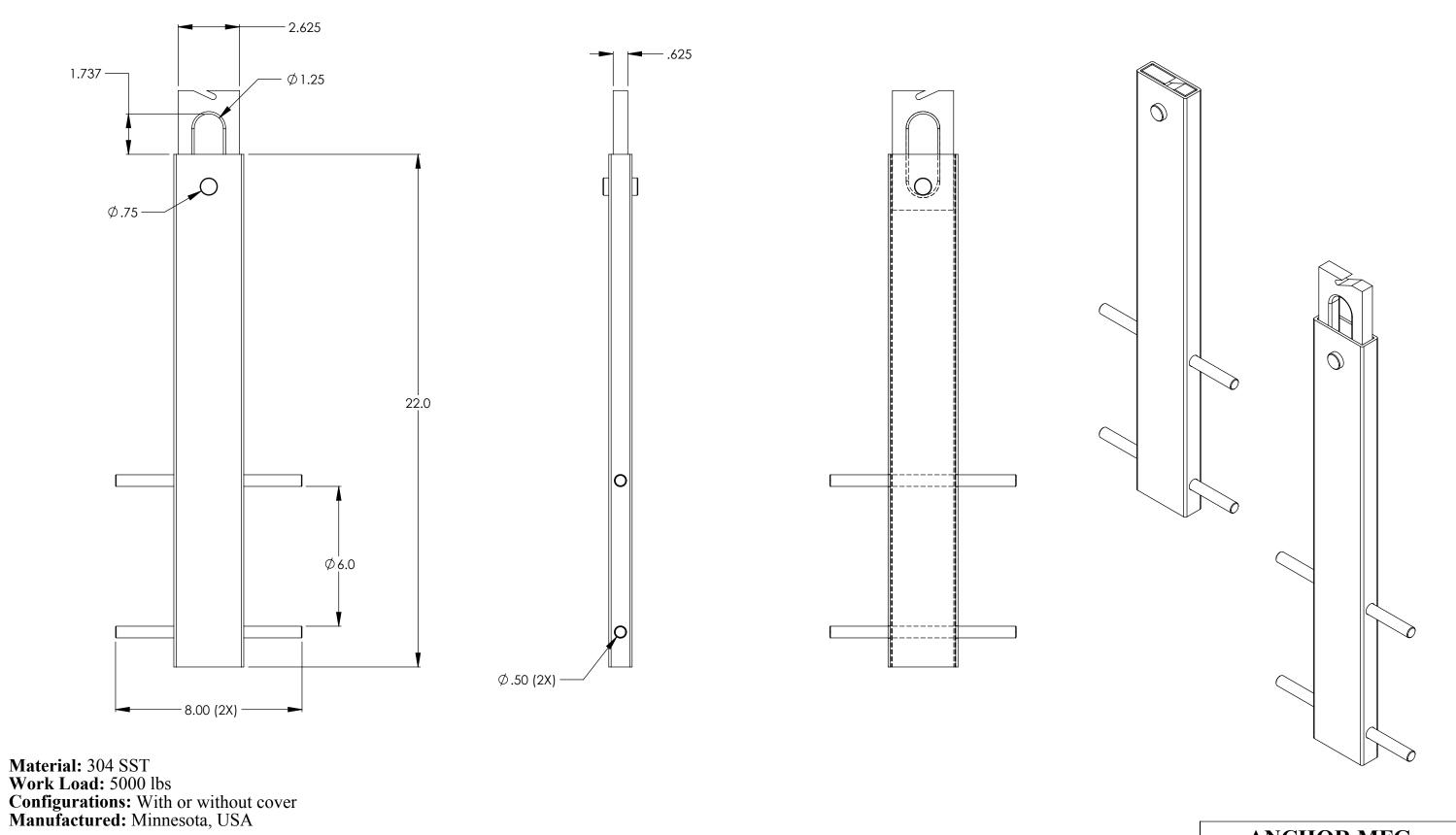
To properly install anchors either an engineer or architect should be consulted to determine the proper depth of concete per soil condition.
