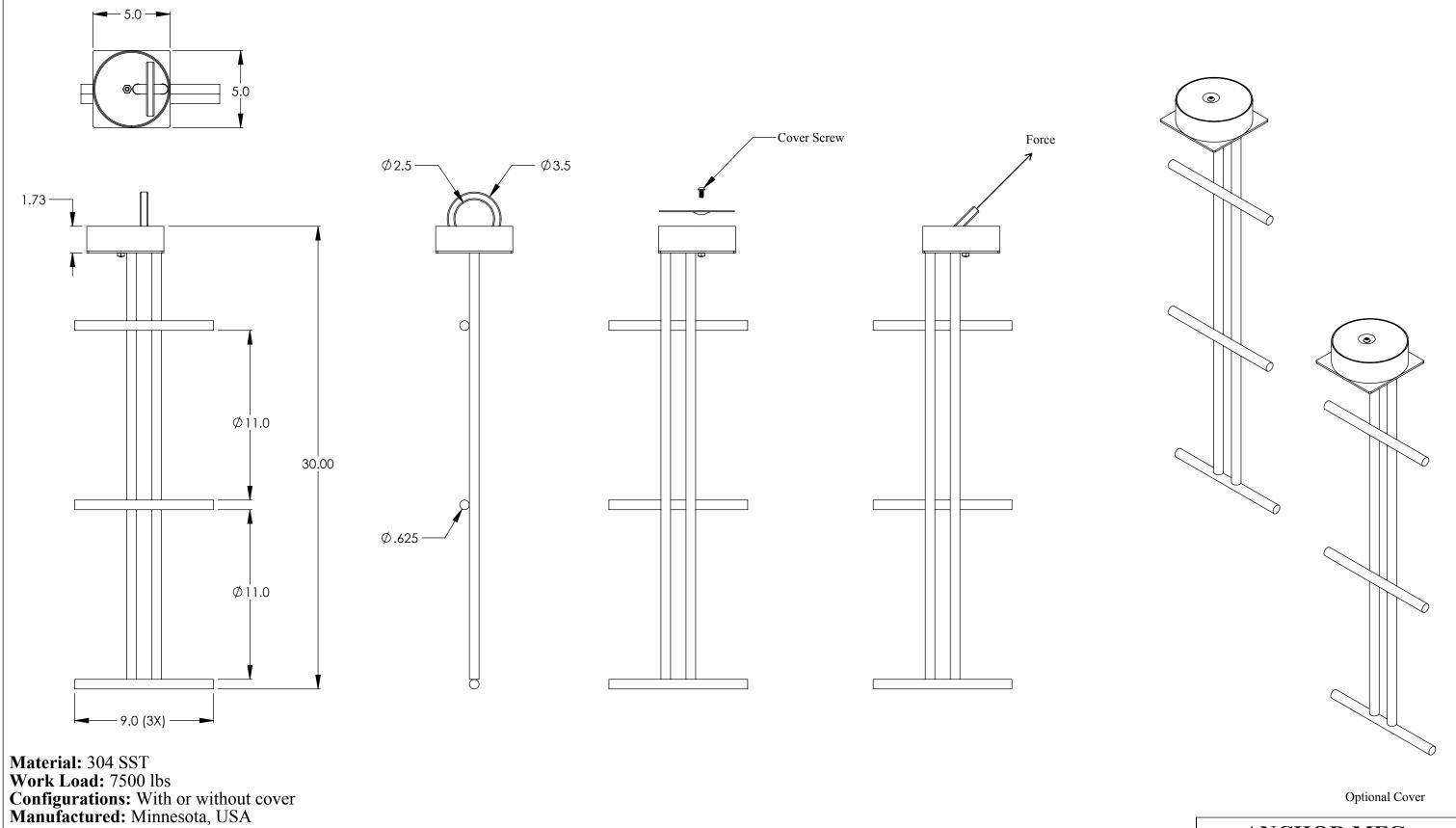
Note: 1. To properly install anchors either a engineer or architect should be consulted to determine the proper depth of concete per soil condition.
